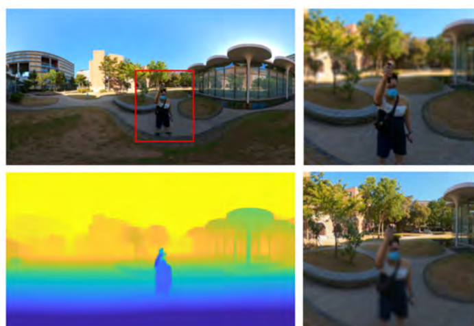
Figure 4: An exterior test scene. The left column is the 360° reference image and the corresponding depth map; the top (bottom) image in the right column is the refocused image of the scene enclosed by the red box in the top-left image on a near (far) focal plane.
