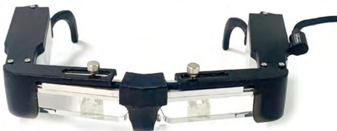
Figure 1: An in-house developed near-eye light field AR display, offering a depth of field ranging from 25 cm to infinity, and enabling users to focus freely on objects within the range [2].
